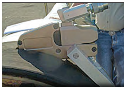
◀ Custom hydraulic torque wrench with reaction paddles for use with a flexible flowline.
