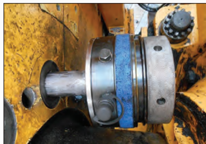
◀ Custom tensioner for removing studs on a stacker reclaimer.
