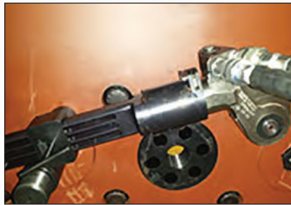
◀ Torque wrench with custom reaction arm for use on fracking equipment maintenance.
